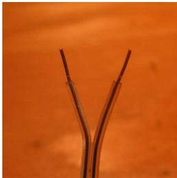
2. Using wire strippers or scissors, strip approximately 1/4 inch of the protective plastic insulator from each wire lead being careful not to cut any of the wires in the process
